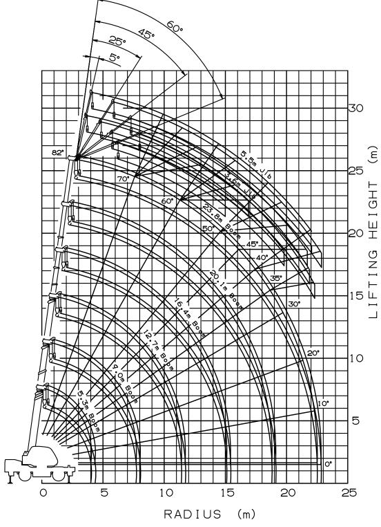
NOTE: 1. The above lifting heights and boom angles are based on a straight (unladen) boom, and allowance should be made for boom deflection obtained under laden conditions.
