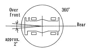
Without outriggers "Over front" operation should be performed within 2 degrees in front of chassis.
